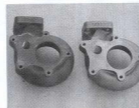
Externally there is not much difference between a large 0.82 A/R (left) and a smaller 0.63 A/R T-3 exhaust housing (right) even though they perform very differently.
