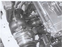
Lisa Kubo's manifold is built to make use of a divided turbine housing to spool a big T61 compressor. It must work well; she is currently the pilot of the world's quickest unibody Honda.
