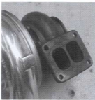
A divided exhaust turbine housing is used on the AEB5 Focus to help spool its monstrous T61 compressor.
