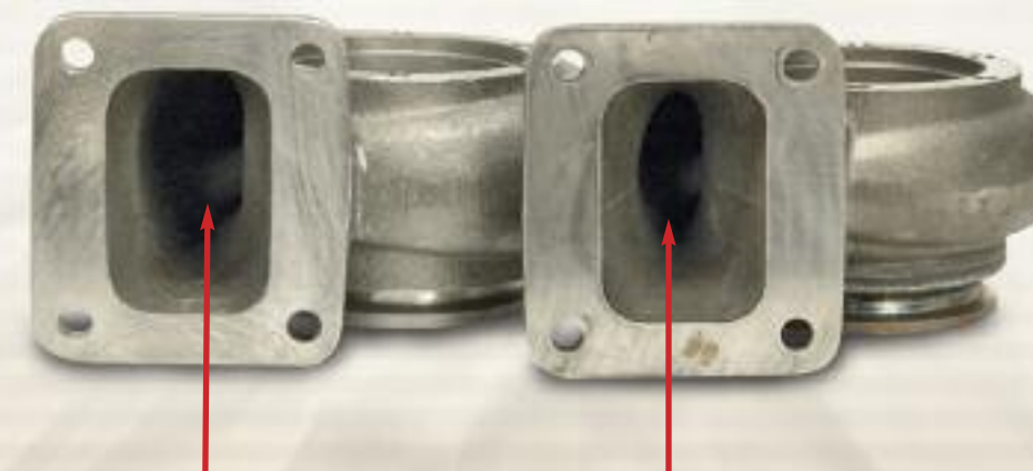
Notice how tight the throat of the volute is on the right turbine housing. The smaller A/R dramatically improves turbine response time.
