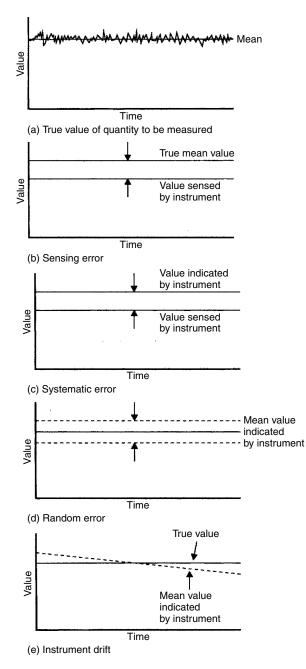
**Figure 20.4** Various types of instrumentation error. (a) True value of quantity to be measured plotted against time – on the same time scale; (b) sensing error; (c) systematic error; (d) random error; (e) instrument drift
