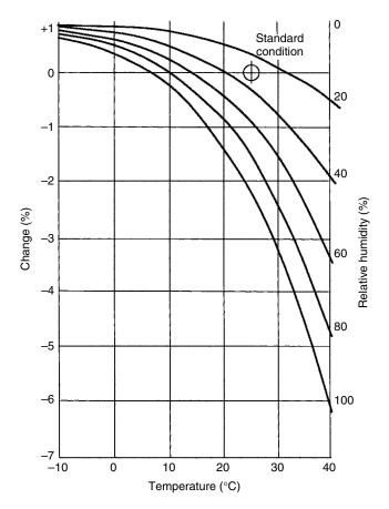
**Figure 12.5** Variation of air charge mass with relative humidity at different temperatures
