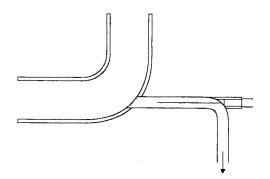
Figure 20.3 Measurement of exhaust gas temperature by suction pyrometer
