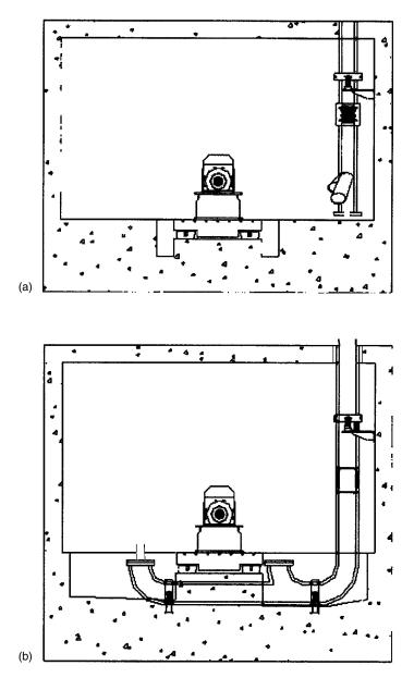
**Figure 6.6** (a) Layout of subfloor exhaust collection duct suitable for left- or right-handed or Vee exhaust configurations and tapping for purge system of subfloor space. (b) Layout of above-floor exhaust dilution duct for collection to vehicle exhaust system and low level purge system
