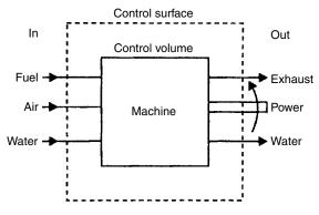
Figure 2.1 An open thermodynamic system
