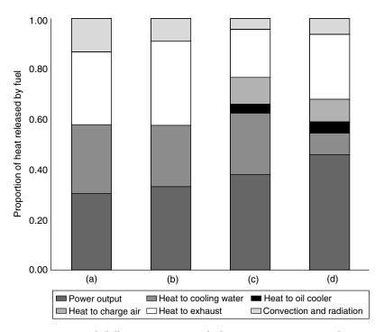
**Figure 13.5** Typical full power energy balances: (a) 1.71 gasoline engine (1998); (b) 2.51 naturally aspirated diesel engine; (c) 200 kW medium speed turbocharged marine diesel; (d) 7.6 MW combined heat and power unit
