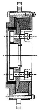
Figure 9.10 Annular type rubber coupling
