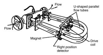
Figure 12.4 Coriolis effect flow meter
