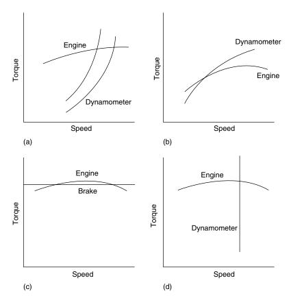
**Figure 11.1** Control modes, engines and dynamometers: (a) position mode stable hydraulic dynamometer; (b) position mode unstable hydraulic dynamometer; (c) position mode, friction brake; (d) position/speed mode; (e) position/torque, governed engine; (f) speed/torque mode; (g) torque/speed mode
