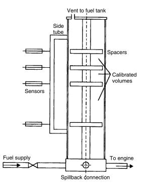
Figure 12.1 Volumetric fuel consumption gauge
