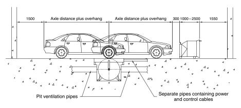
**Figure 18.4** A single roll set  $(2 \times 2)$  chassis dynamometer plus road speed following cooling fan, within a cell sized to test rear and front wheel drive cars (AVL Zöllner)
