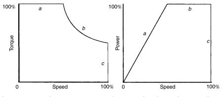
**Figure 8.14** Performance curve shapes of electrical motor-based dynamometers
