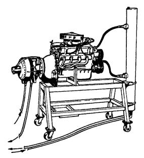
Figure 4.1 Portable engine test stand
