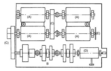
**Figure 18.2** Schematic plan view of four roller  $(2 \times 2 = single driven axle)$ emission chassis dynamometer of late 1980s design. (A) Four 500-mm rollers; (B) selectable flywheel set; (C) belt drive; (D) d.c. motor fitted with shaft encoder; (E) disk brake for vehicle loading
