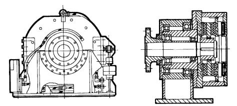
Figure 8.12 Water-cooled friction brake used as a dynamometer
