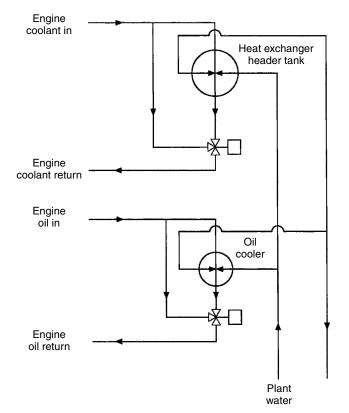
Figure 6.3 Circuit diagram of unit in Fig. 6.2
