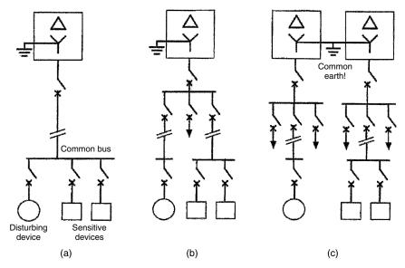
**Figure 10.8** Different power connection layouts ranging from poor (a) to recommended (c)
