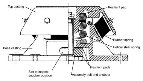
Figure 3.9 Combined spring and rubber flexible mount
