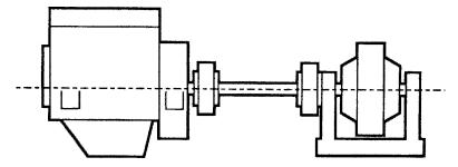
Figure 9.1 Simple form of dynamometer/engine drive line
