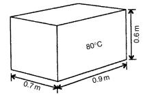
**Figure 5.1** Simplified model of exampled 100 kW engine, for analysis of heat transfer to surroundings
