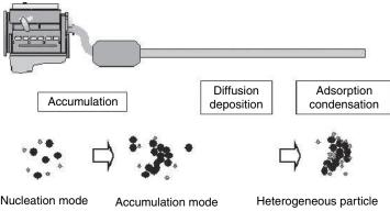
Figure 16.2 Phases of particle formation
