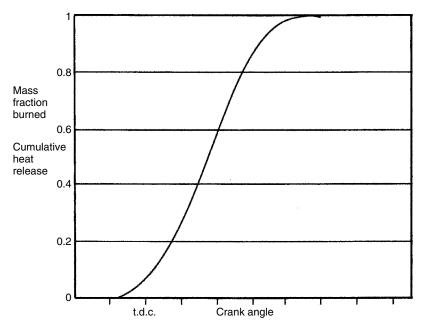
Figure 14.6 Mass fraction burned plotted against crank angle
