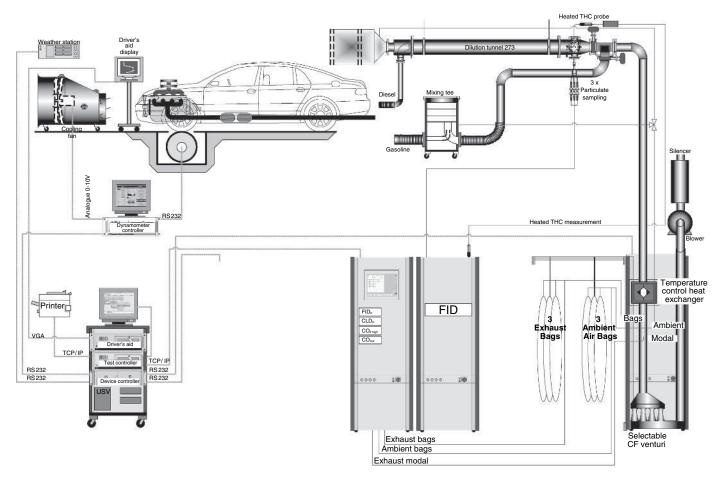
Figure 16.8 The major components of a Euro 3 CVS system
