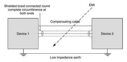
**Figure 10.3** Recommended method of connecting shielded cable between devices to prevent EMI and ground loop corruption of signals
