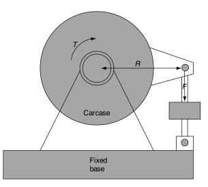
**Figure 8.2** Diagram of trunnion-mounted dynamometer measuring torque with a load cell
