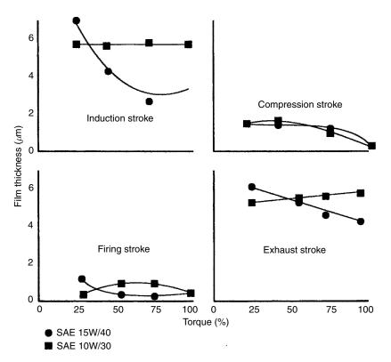
**Figure 17.2** Oil thickness between ring and cylinder liner during four-stoke operation
