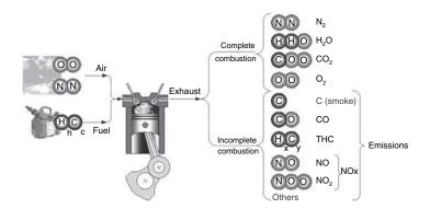
Figure 16.1 Gaseous components of combustion processes
