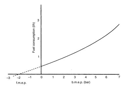
Figure 13.8 Willan's line for a diesel engine
