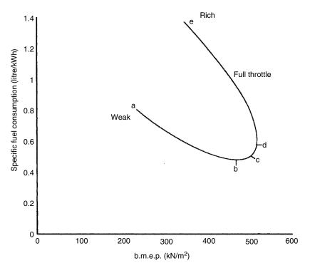
Figure 14.1 Hook curve for gasoline engine
