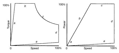
Figure 8.15 Performance curve shapes of an eddy-current dynamometer
