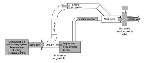
**Figure 5.12** AVL dynamic combustion air pressure control system. Example flows shown at engine idle condition
