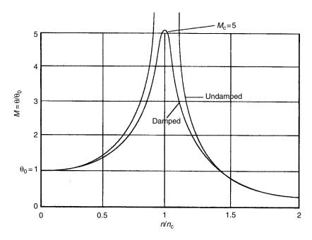
**Figure 9.3** Relationship between frequency ratio, amplitude and dynamic amplifier M
