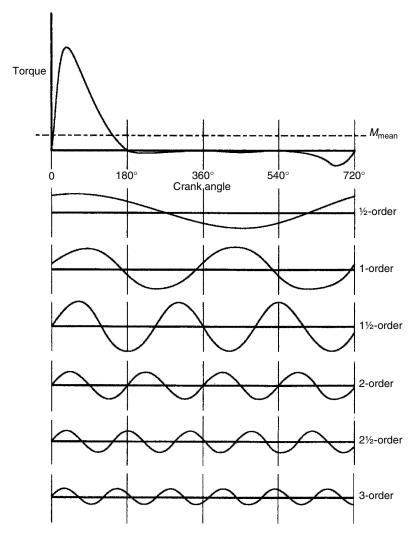
**Figure 9.4** Harmonic components of turning moment, single cylinder fourstoke gasoline engine
