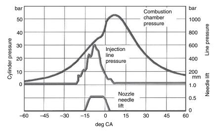
Figure 14.12 Typical engine indicating display parameters
