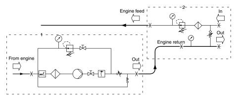
**Figure 7.5** Regulation of engine supply and return pressures within dotted lines (1) is the fuel return pressure control and (2) the fuel feed to the engine from the fuel consumption measurement system (AVL List)
