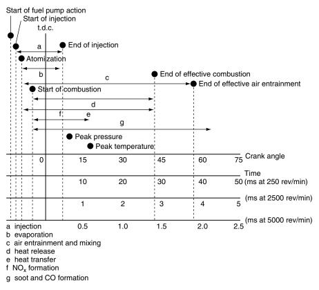
Figure 14.7 Time scale of diesel combustion process
