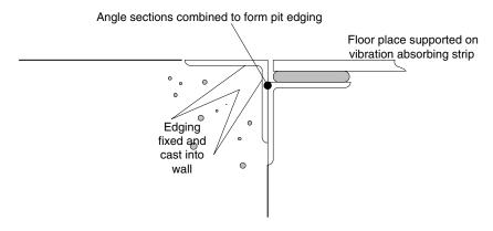
**Figure 18.6** Section through one form of pit edging required to support pit flooring
