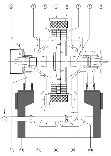
**Figure 8.3** Schenck, dry gap, disc type eddy-current dynamometer 1, rotor; 2, rotor shaft; 3, coupling flange; 4, water outlet with thermostat; 5, excitation coil; 6, dynamometer housing; 7, cooling chamber; 8, air gap; 9, speed pick-up; 10, flexure support; 11, base; 12, water inlet; 13, joint; 14, water outlet pipe
