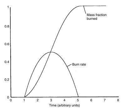
Figure 14.3 Combustion in a constant volume bomb calorimeter
