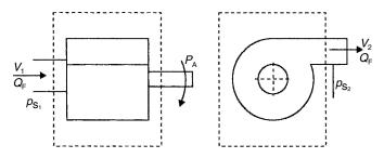
Figure 5.8 Centrifugal fans as an open system
