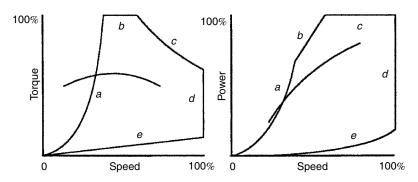
**Figure 8.13** Engine torque curves plotted on hydraulic dynamometer torque curves
