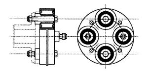
Figure 9.8 Rubber bush type torsionally resilient coupling
