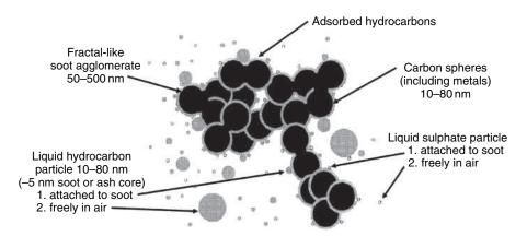
Figure 16.4 Schematic representation of diesel particles (Kulijk–Foster)
