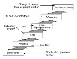
Figure 14.11 Typical workflow process through combustion analysis
