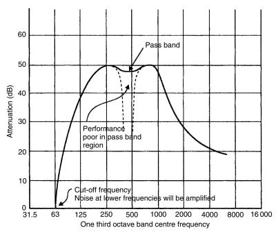
Figure 3.16 Sample performance of a reactive muffler
