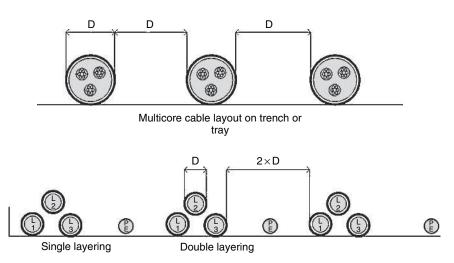
Figure 10.7 Recommended spacing and layout of power cables
