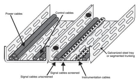
Figure 10.6 Segmented trays or trunking and separation of types of cable
