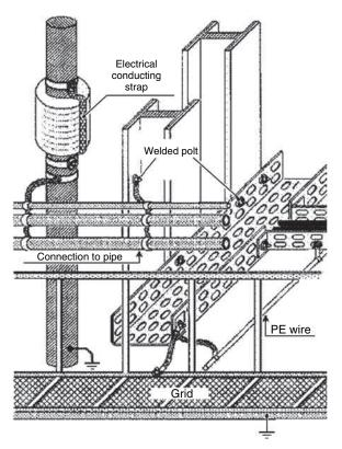
Figure 10.5 Continuous linked network of all ground potentials
