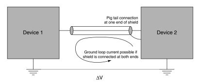
**Figure 10.2** Recommended method of connecting shielded cable between devices to prevent ground loop current distortion of signals
