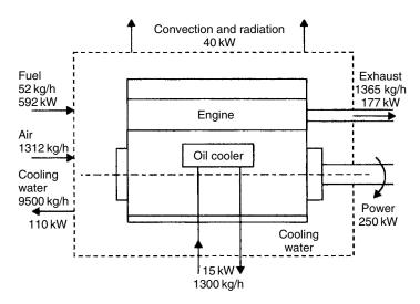
**Figure 13.6** Control volume, 250 kW diesel engine showing energy and fluid flows
