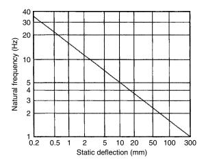
Figure 3.4 Relationship between static deflection and natural frequency
