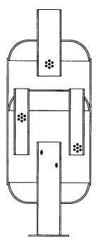
Figure 3.15 Exhaust resonator or reactive muffler
