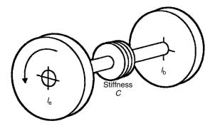
Figure 9.2 Two mass system (compare with Fig. 9.1)
