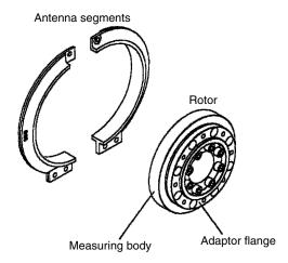
Figure 8.5 Shaft-line components of a torque flange
