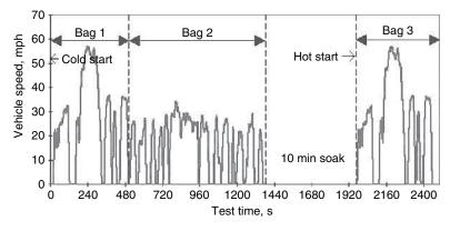
Figure 16.11 EPA urban dynamometer driving schedule
