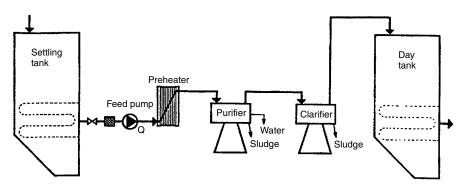
Figure 7.3 Fuel supply and treatment system for residual fuel oil
