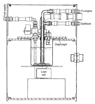
Figure 12.2 Gravimetric, direct weighing, fuel gauge
