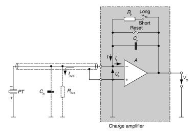
Figure 14.10 Basic charge amplifier circuit (AVL List)
