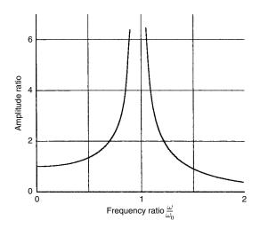
**Figure 3.5** Relationship between frequency and amplitude ratio (transmissibility) undamped vibration
