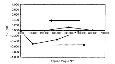
Figure 8.6 Dynamometer calibration error as percentage of applied torque
