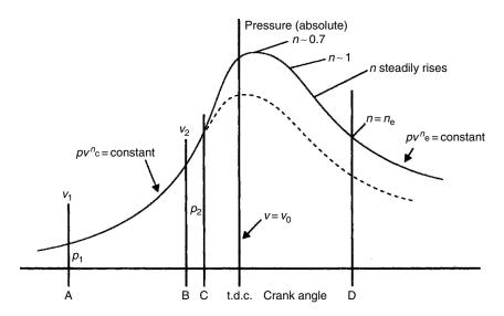
**Figure 14.4** *Pressure–crank angle diagram showing derivation of mass fraction burned*
