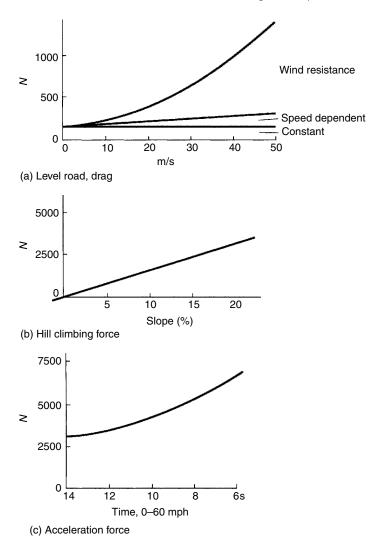
**Figure 18.1** Vehicle drag: saloon of laden weight 1600 kg (a) level road performance; (b) hill climbing; (c) acceleration force
