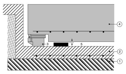
**Figure 3.11** Seismic block or cast bedplate (not shown) (4) mounted on air springs (3) within a shallow concrete pit (2) on consolidated subsoil (1). When the air supply is off the self-levelling air springs allow the block to settle on support blocks (5) the rise and fall typically being 4 to 6 mm. Maintenance access to the springs is not shown
