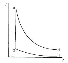
Figure 13.1 Air standard cycle
