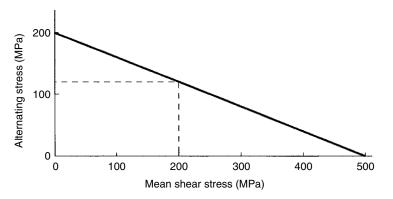
Figure 9.6 Goodman diagram, steel shaft in shear
