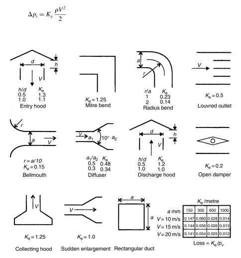
Figure 5.3 Pressure losses in components of ventilation systems
