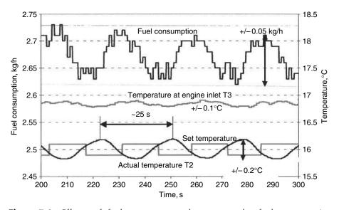
**Figure 7.6** Effects of fuel temperature changes on the fuel consumption measurement values. T2 is the controlled outlet of the fuel conditioning device superimposed on the step demand changes. T3 is the temperature at the engine inlet. The difference between the two is due to system damping (AVL List)
