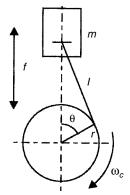
Figure 3.2 Connecting rod crank mechanism: unbalanced forces
