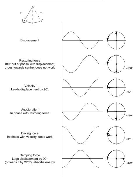
Figure 3.12 Diagram of phase relationship of vibrations
