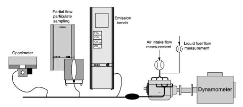
**Figure 16.6** Typical emission plant used in ISO 8178 engine emission cycles (diesel)
