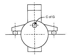
Figure 3.3 Engine carried on four flexible mountings
