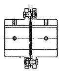
Figure 9.7 Multiple steel disc type flexible coupling
