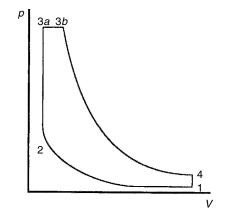
Figure 13.2 Limited pressure cycle
