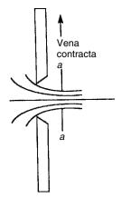
Figure 12.7 Flow through a sharp-edged orifice
