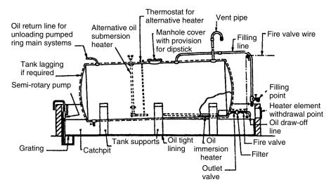
**Figure 7.1** Typical above ground bunded fuel tank with fittings
