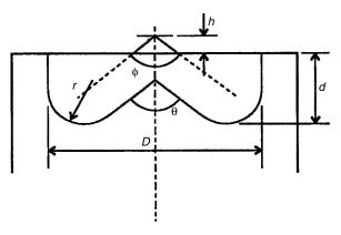
Figure 15.3 Diesel engine combustion system
