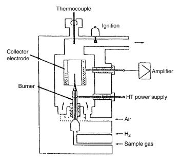
Figure 16.7 Flame ionization detector
