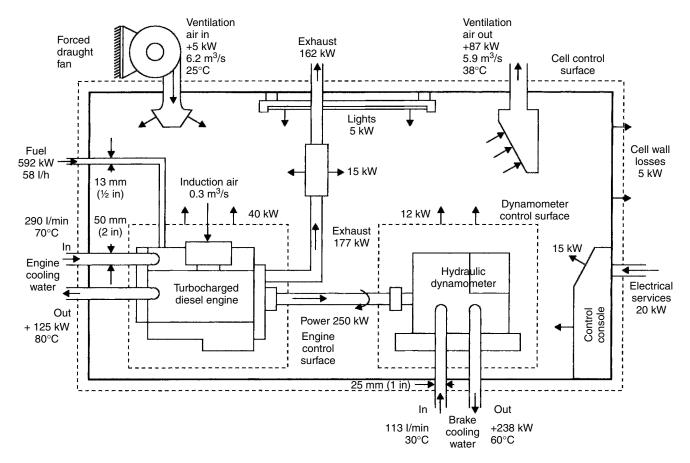
Figure 6.4 Energy balance and energy flow diagram for example 250 kW cell
