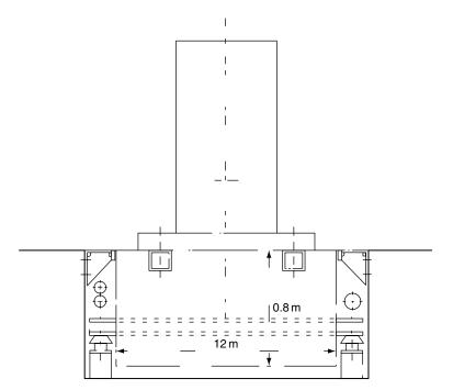
Figure 3.8 Spring-mounted seismic block
