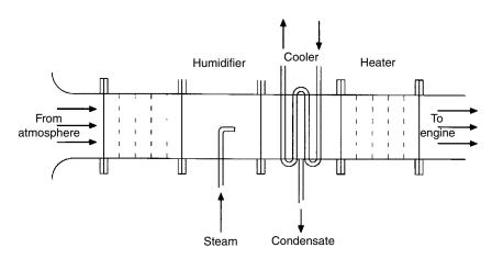
Figure 5.11 Schematic of typical combustion air system contents
