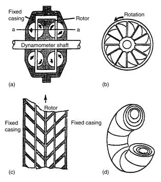
**Figure 8.9** Hydrokinetic dynamometer, principle of operation: (a) section through dynamometer; (b) end view of rotor; (c) development of section a–a of rotor and casing; (d) representation of toroidal vortex
