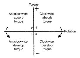
Figure 8.8 Dynamometer operating quadrants
